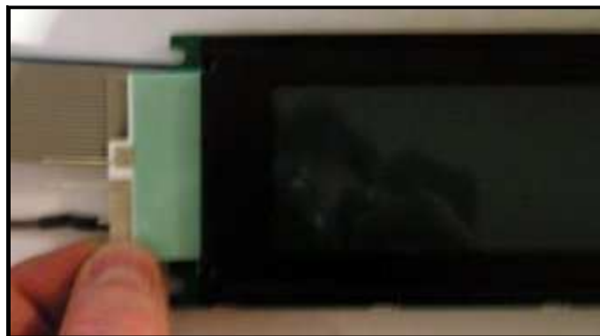
Inserting the EL-panel into the LCD(wrong EL side!)
