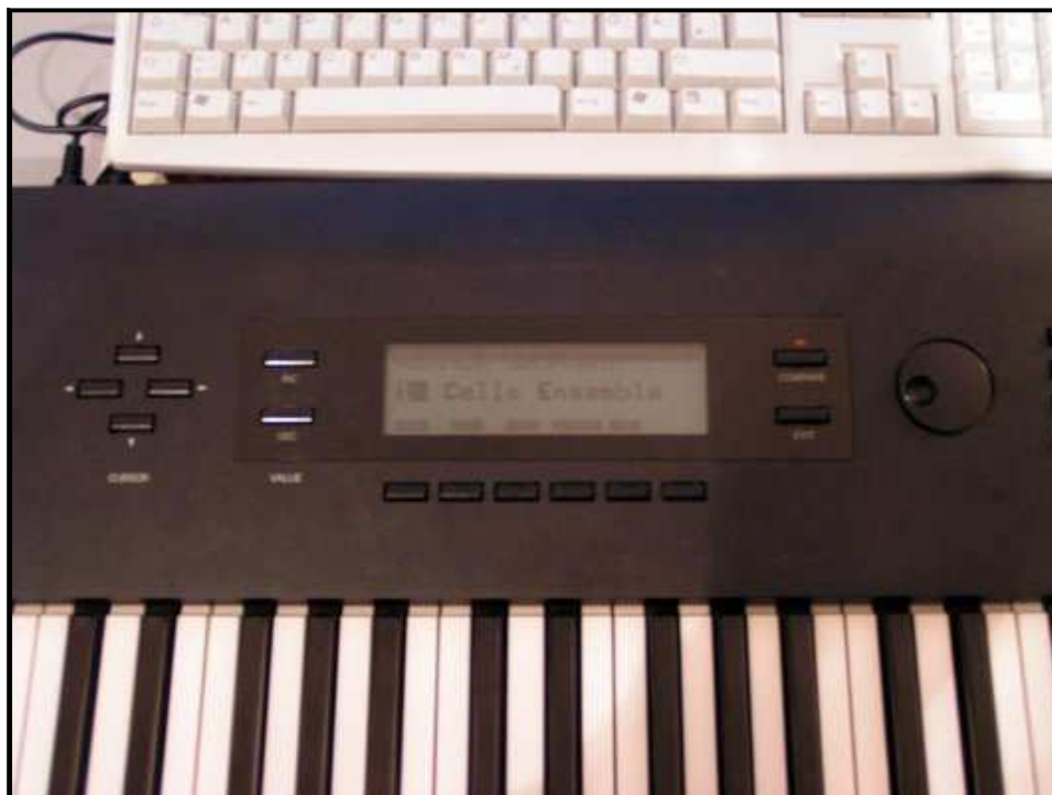
Display of a Wavestation EX with a dead backlight
