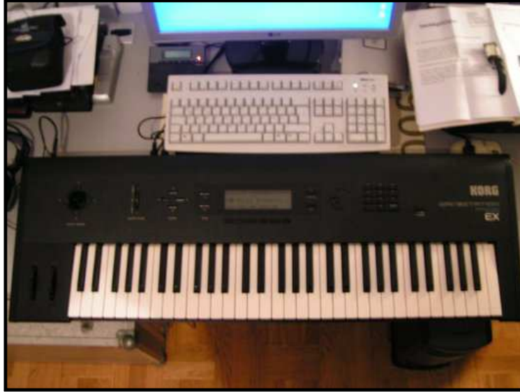
Wavestation EX with a dead EL-panel
