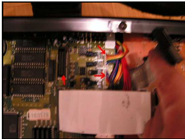
Remove small flatcable and 2 connectors
