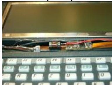
7. Open the two palmtop halves as much as possible and reattach the hinge tube. Press firmly, and take care not to crimp any cables. The inverter with its coil should fit nicely into the tube. If not, rearrange the cables and inverter a bit, so that it fits.
