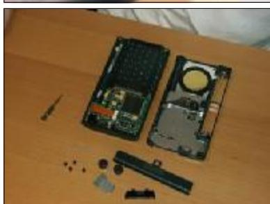
8. Check to see if the battery contacts in the bottom shell came out of their mountings and if so, press them back into position.
