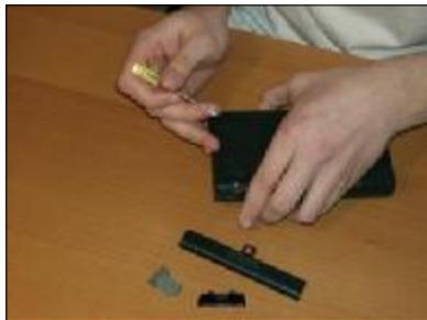
4. Unscrew the four Torx-6 screws under the rubber feet.
