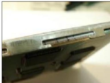
3. Open the sandwich: separate the LCD from the circuit board, take care that the white rubber strips remain on the LCD and take care not to damage the yellow ribbon cable between LCD and circuit board. If the white rubber bands don't stick on the LCD, you may have problems when reassembling the screen. See below.
