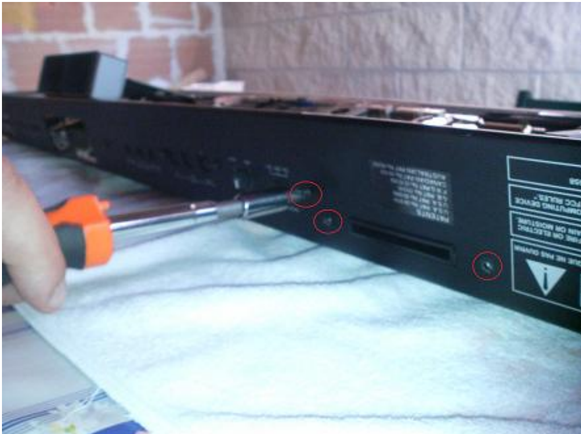
REMOVE THE 3 SCREWS CLOSE TO THE OTHER SLOT ON THE RIGHT
