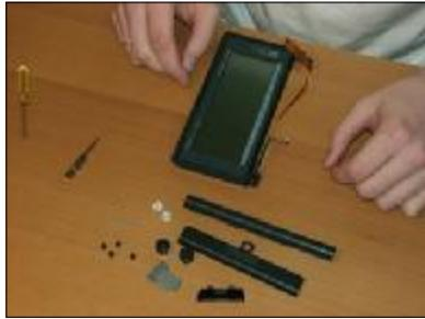
12. Remove the display cover. Use a small knife or screw driver to peel the cover off in one edge, then pull it off entirely. This needs a bit of force, but can easily be reattached afterwards. Take care not to scratch the screen!
