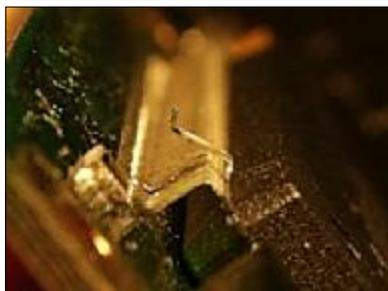
2. Pin 1 of the inverter chip on the inverter module is already lifted, but connected to + polarity (= backlight permanently enabled) the circuit board by a small wire that it can be tested on
