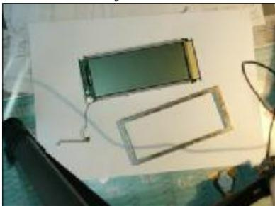
2. Apply some markings with a sharp pen on the white rubber and on the side of the circuit board, so you can later adjust both into their exact relative horizontal position they are now in. Apply more than one such markings on one side, so you may later see a few of them even if the metal frame is attached again.
