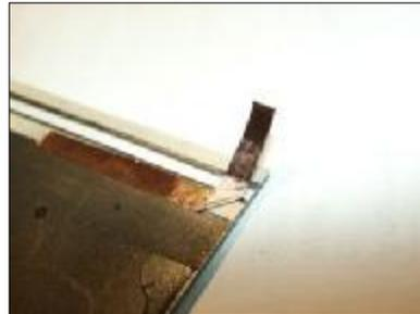
4. Insulate the other EL contact, where the copper foil crosses it, using adhesive tape!
