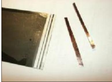
3. Clean the metal contacts of the EL foil carefully with an eraser or another kind of rubber, remove the protection layer of one of the copper foils and attach the copper foil firmly to the EL contact as the following pictures show:
