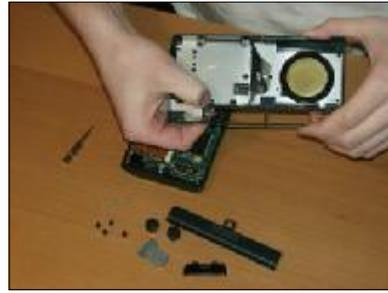
9. You now see the motherboard lying in the keyboard shell. Detach the screen cable from its motherboard connector using your fingernail to slide the top restraining clasp toward the cable. Once the screen cable is disconnected, you can simply take out the motherboard.
