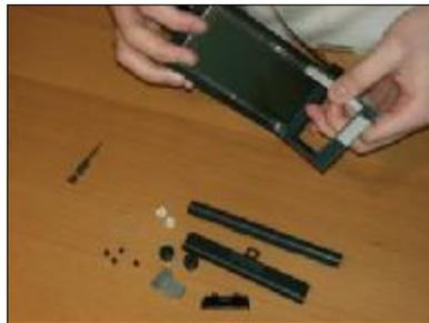
13. Unscrew the four Torx-6 screws of the screen
