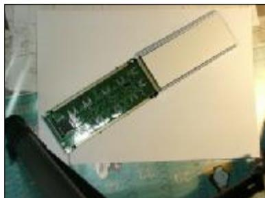
**Take much care of the yellow ribbon cable! If you apply too much force to it, that can lead to missing horizontal lines after the upgrade process. This is not repairable!**
