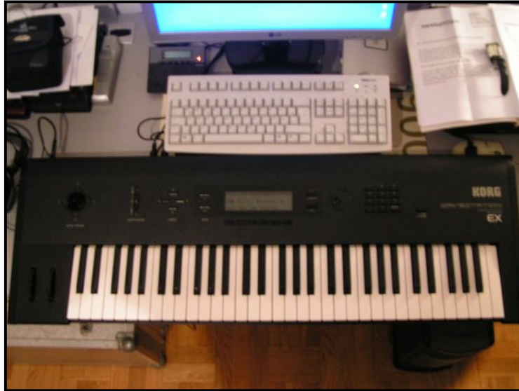
Wavestation EX with a dead EL-panel
