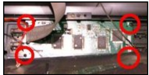
Screws of the Optrex DMF5005N
