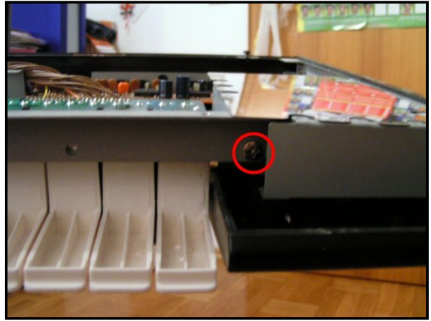
Position screws on the right
