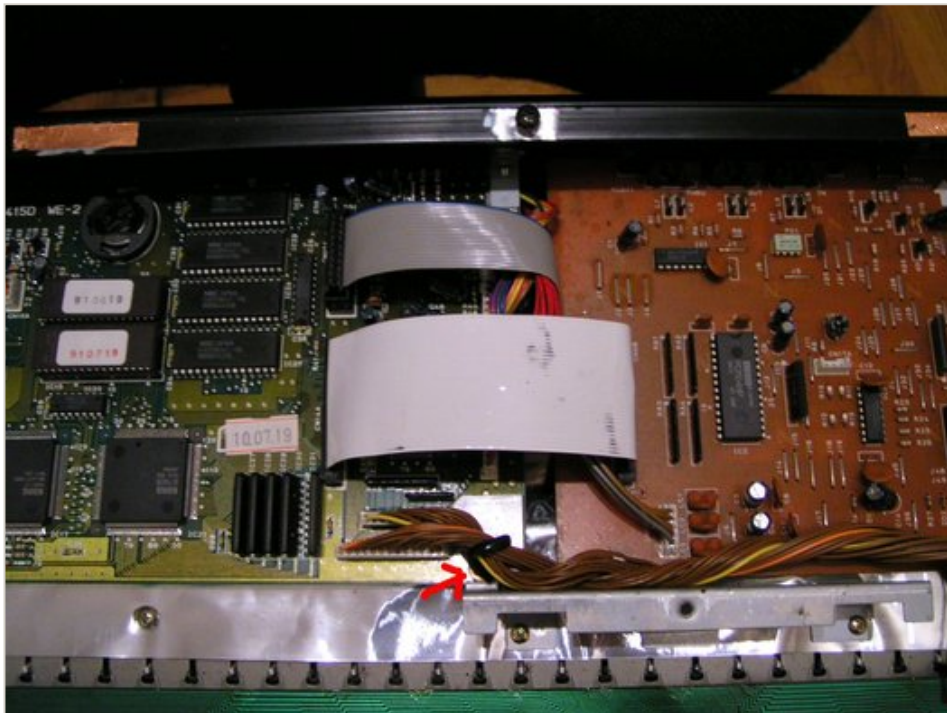
Right side of the mainboard KLM-1415D
