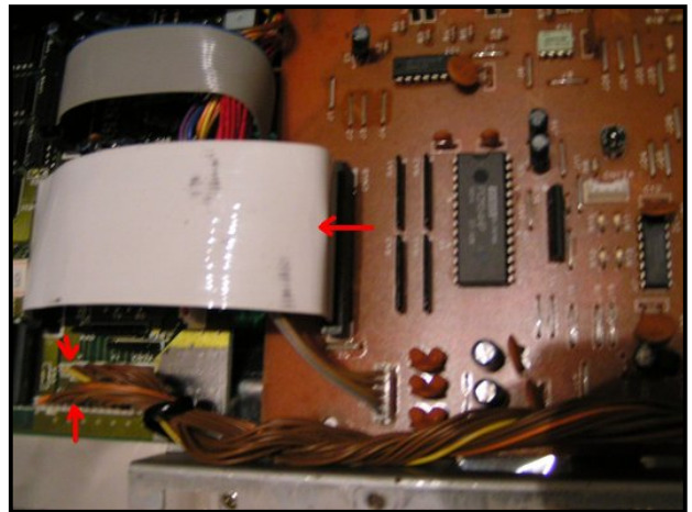
Remove big flatcable and 2 connectors
